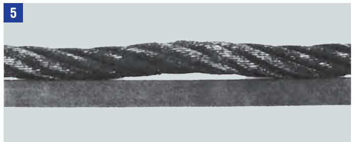
Flattened wire rope caused by over-ride
