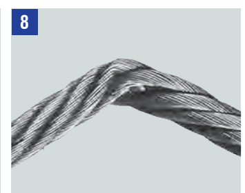
Kind caused by mechanical impact
