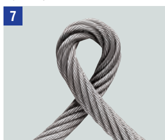
Bend caused by a pinched rope sling
