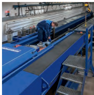
Pull Test Facility 6,000 kN
