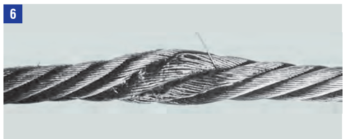
Bend caused by a pinched rope sling
