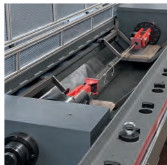
Pull Test Facility 800 kN
