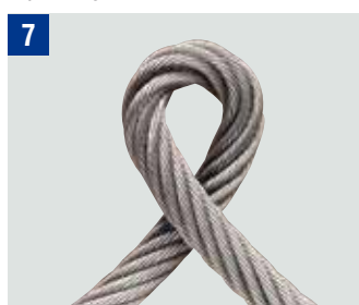
Bend caused by a pinched rope sling
