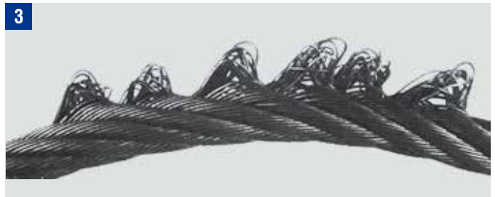
Through corrosion and wear heavy loose strand
