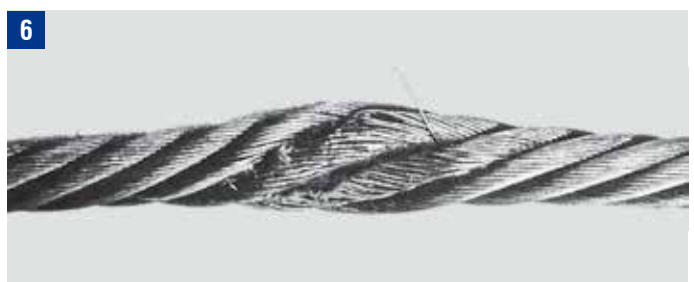
Bend caused by a pinched rope sling
