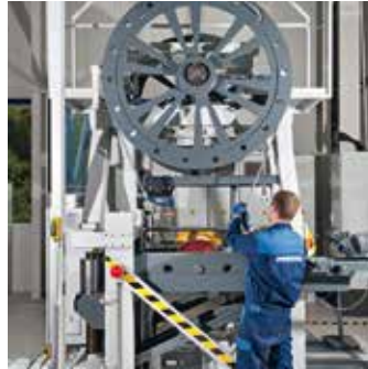
Test Facility for Determining Bending Fatigue
