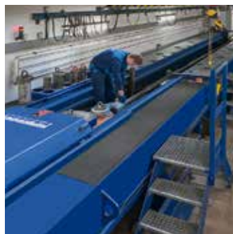
Pull Test Facility 6,000 kN
