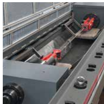
Pull Test Facility 800 kN
