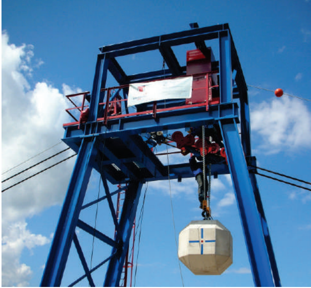
Tests following certification guidelines are carried out using standardized blocks to simulate impacts up to more than 5000 kJ.
