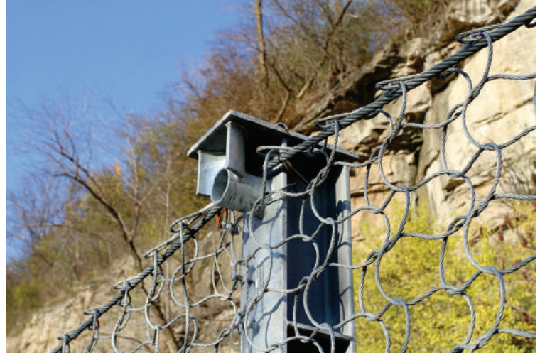
The rope guidances on the posts and base plates are integrated and designed to be robust, giving the ropes smooth surfaces to glide over during an impact to help minimize fatigue. There is no assembly required.
