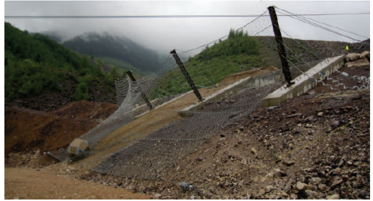
During the impact, the majority of the energy is absorbed during the initial contact with the upper section of the structure, but the projectile is allowed to progress through the system to the bottom portion of the net.
