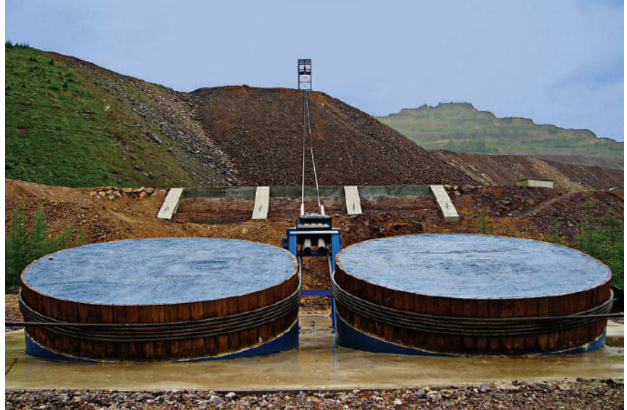
The inclined test facility from Trumer is one of the largest and most modern in the world and can accommodate a large variety of types of fences as well as earth dams.
