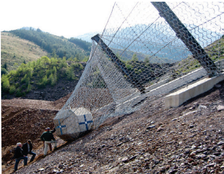
A completed Maximum Energy Level test for a 5000 kJ rockfall catchment fence.
