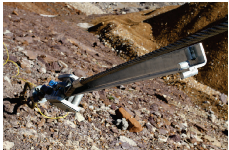
A new generation of brake elements uses a roller to deform an angled steel strip in a very efficient and compact manner.
