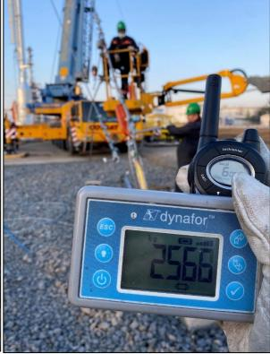
Design Tension tolerance: +/- 10 %
