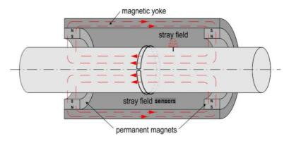
The measurement instrumentation is designed to detect local faults (LF) and loss of metallic area (LMA). Local faults are generally wire breaks while loss of metallic area is generally categorized as a gradual or extended loss in cross-sectional area due to corrosion, wear, or other wire rope deterioration mechanisms.
